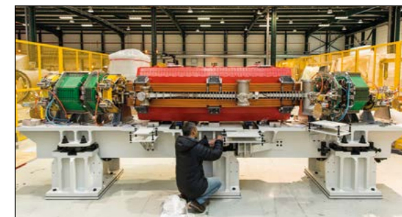
The first of 16 cells of the SESAME storage ring, assembled for testing at CERN in late March, with components constructed in SESAME members and observers: quadrupoles (green) – Spain and Turkey; dipoles (red) – UK; sextupoles (yellow) – Cyprus and Pakistan; sextupole coils – France; vacuum chambers – Germany; girders – Spain. In addition, there are: dipole power supply – Italy; controllers and corrector power supplies – Switzerland; quadrupole and sextupole power supplies – Israel. (Image credit: CERN-PHOTO-201503-059-31.)
