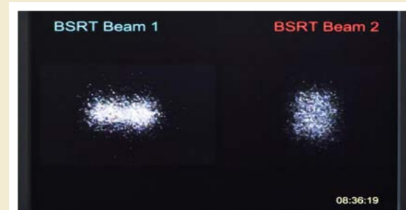
Early in the proceedings on 3 June, cameras record the screens of the beam synchrotron-radiation telescopes at point 4: beam 1 on the left, beam 2 on the right. (Image credit: CERN-PHOTO-201506-125-59.)
