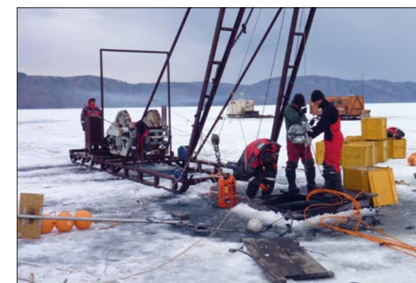
Assembling strings of optical modules. (Image credit: INR RAS.)
