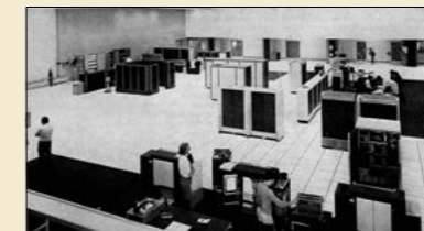
Part of the large hall of the new computer centre. It houses the CDC 7600 (seen in the upper left-hand corner) and a CDC 6400, which serves as a front-end machine channelling computing to and from the 7600. (Image credit: CERN 135.8.72.)
