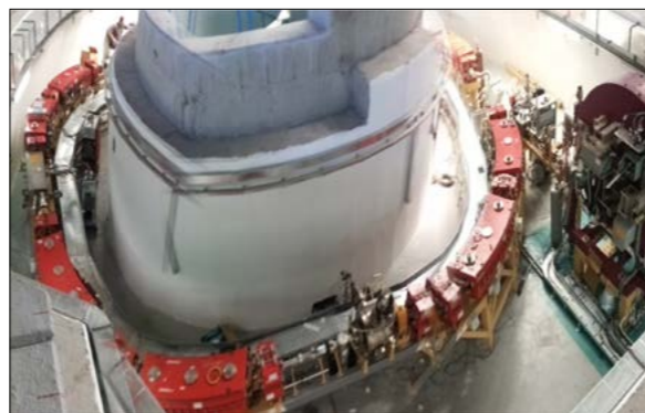
The SESAME booster synchrotron, built using components from BESSY I, pictured here without the shielding roof. It is now the highest-energy accelerator in the Middle East. (Image credit: SESAME.)
